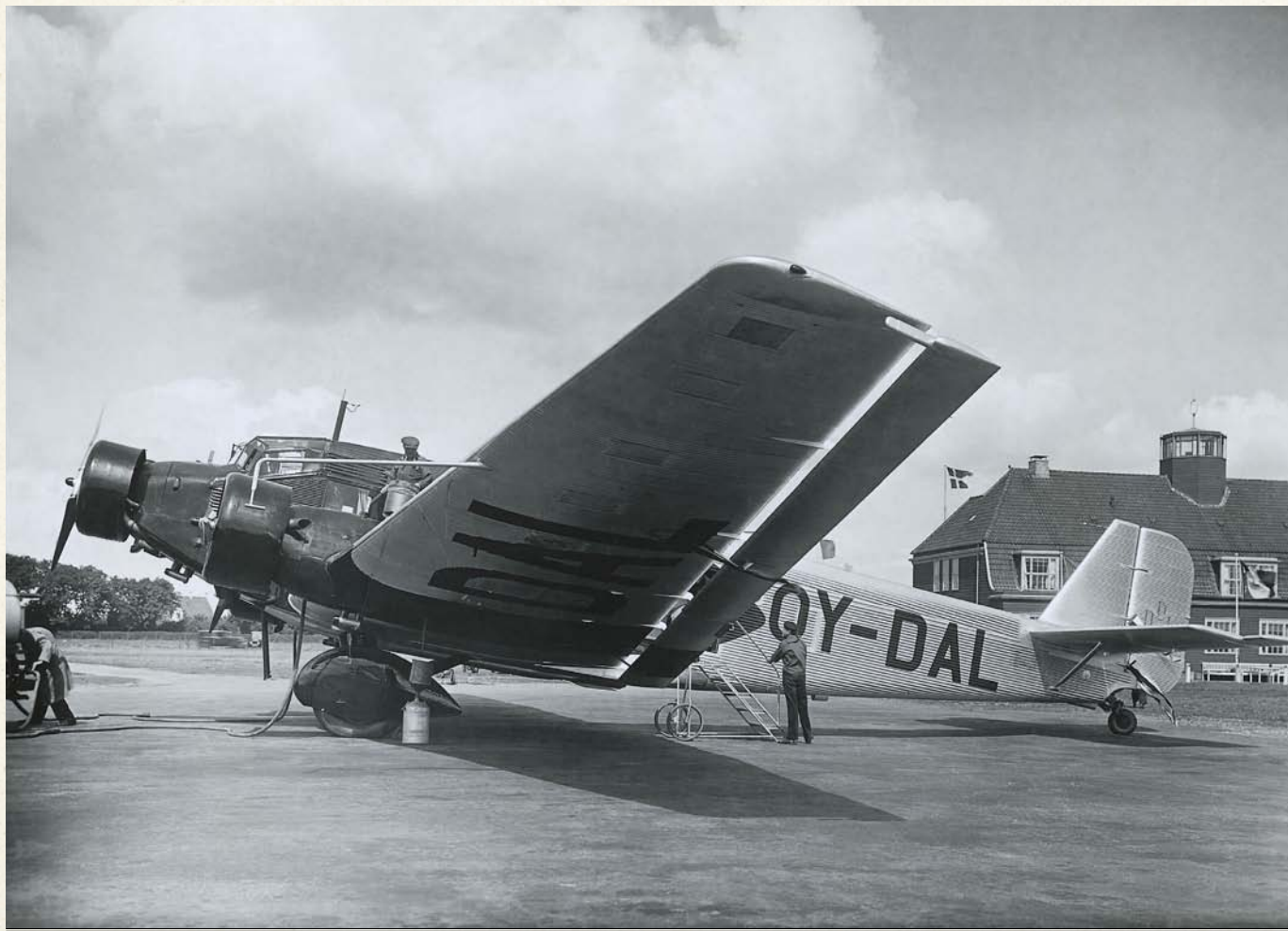
THE TANTE JU WAS THE LAST OF THE JUNKERS' DESIGNS TO USE THE COMPANY'S DISTINCTIVE CORRUGATED-METAL SKINNING
