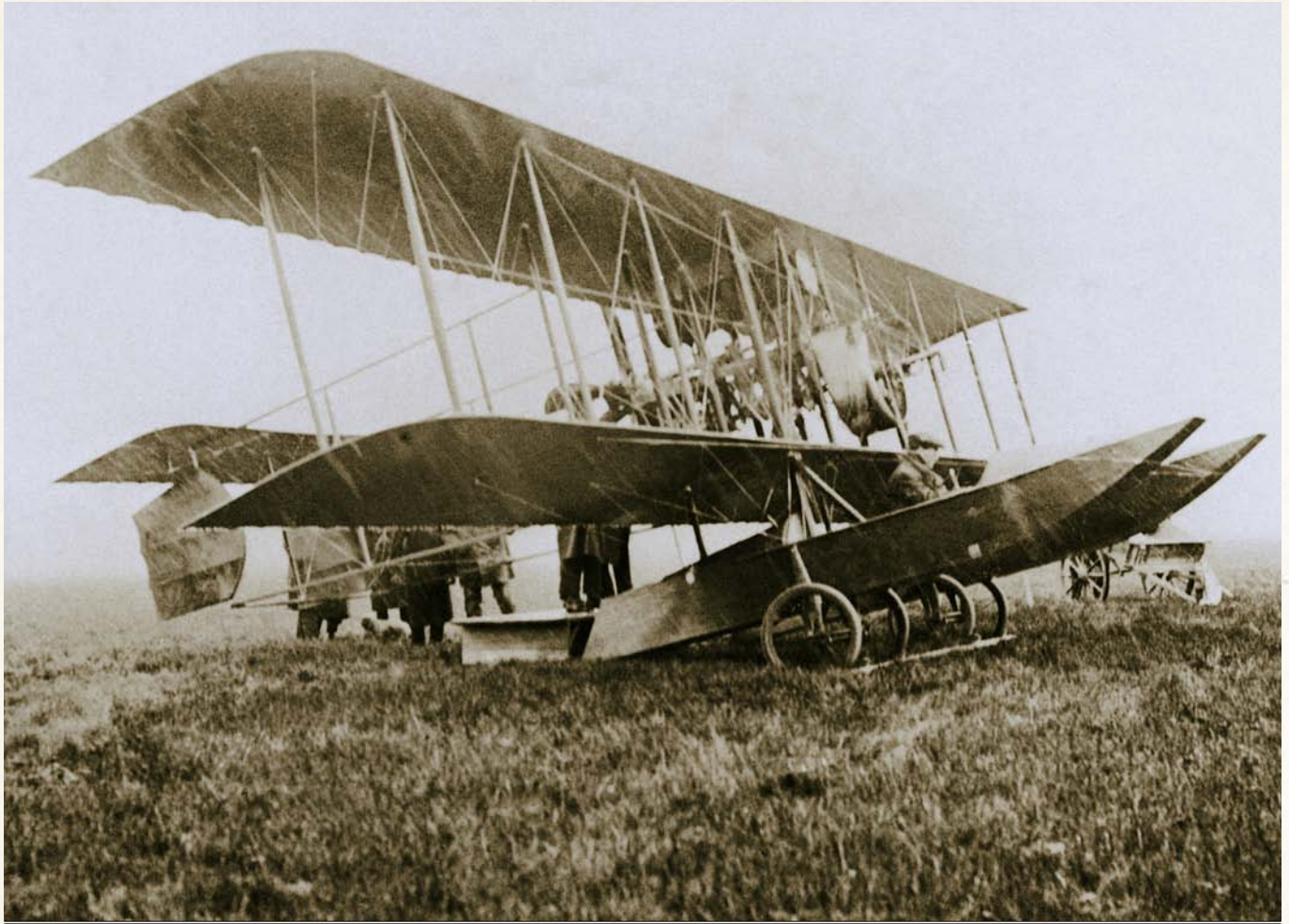
THE RADLEY-ENGLAND WATERPLANE WAS FIRST FLOWN AS A LANDPLANE WITH A TEMPORARY WHEELED UNDERCARRIAGE
