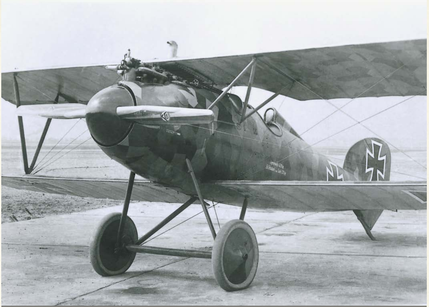
THE STREAMLINED ALBATROS D.V WAS ARMED WITH TWO SYNCHRONIZED, FORWARD-FIRING SPANDAU MACHINE GUNS
