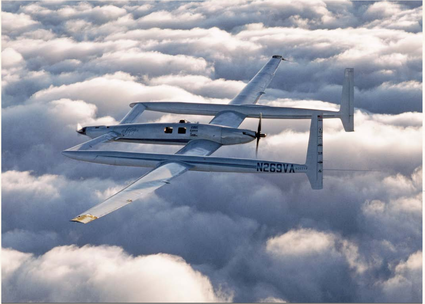
VOYAGER'S 17 FUEL TANKS CARRIED 7,011LB OF FUEL – MORE THAN 72 PER CENT OF ITS GROSS WEIGHT AT TAKE-OFF
