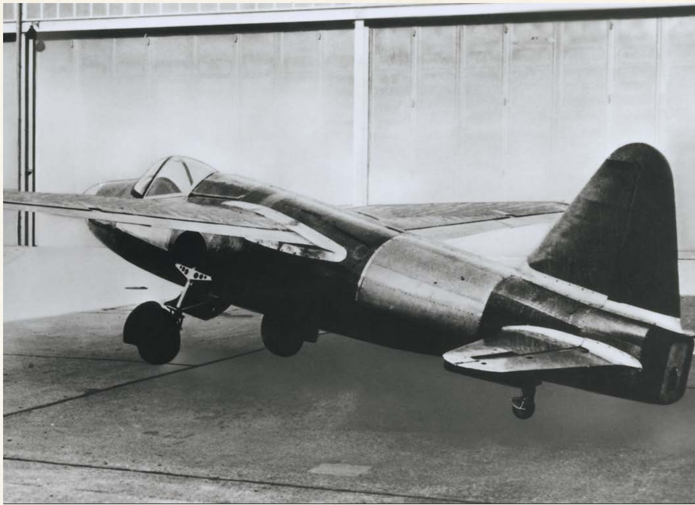
THE He 178 WAS THE FIRST AEROPLANE EVER TO FLY ON TURBOJET POWER ALONE
