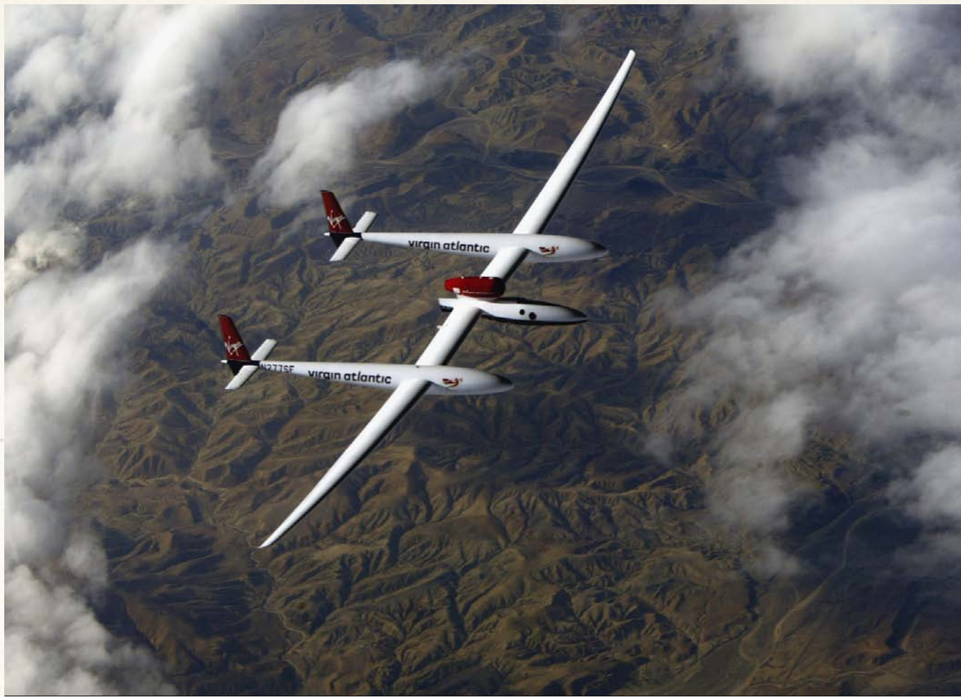
GLOBALFLYER'S SINGLE WILLIAM'S FJ44-3 JET ENGINE IS SET ABOVE THE TINY, CENTRALLY-LOCATED, PRESSURIZED COCKPIT
