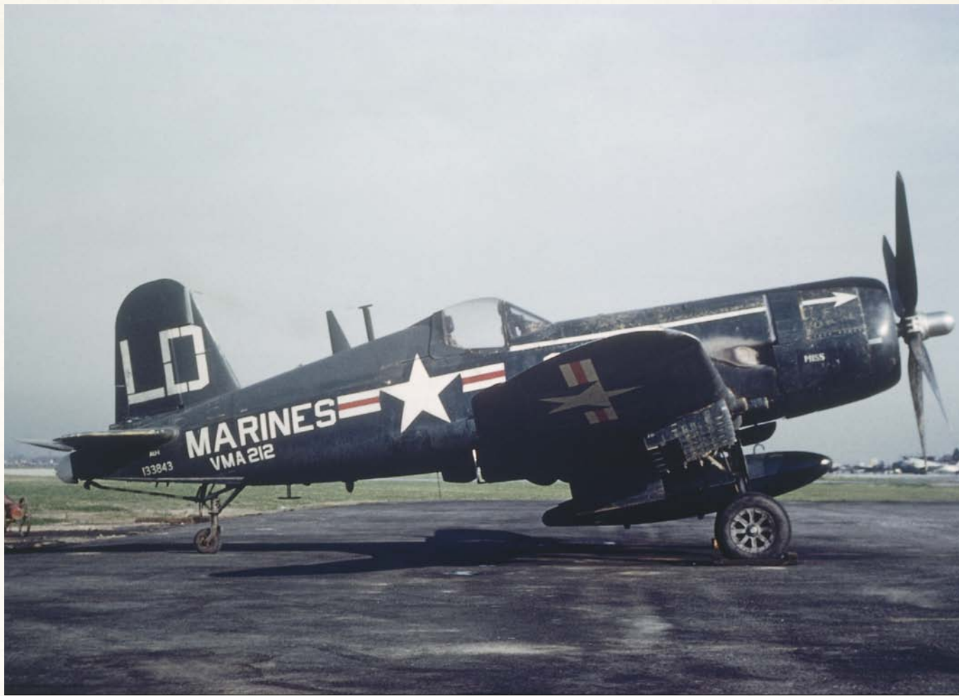
THE F4U HAD A DISTINCTIVE INVERTED-GULL WING THAT ALLOWED A SHORTER UNDERCARRIAGE TO BE USED
