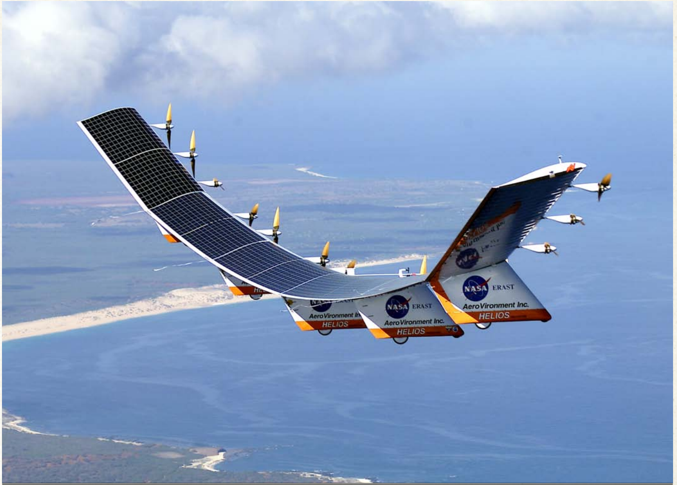
THE CURIOUS-LOOKING FLYING WING, HELIOS, WAS BUILT PRIMARILY OF COMPOSITE MATERIALS AND ASSEMBLED IN SIX SECTIONS
