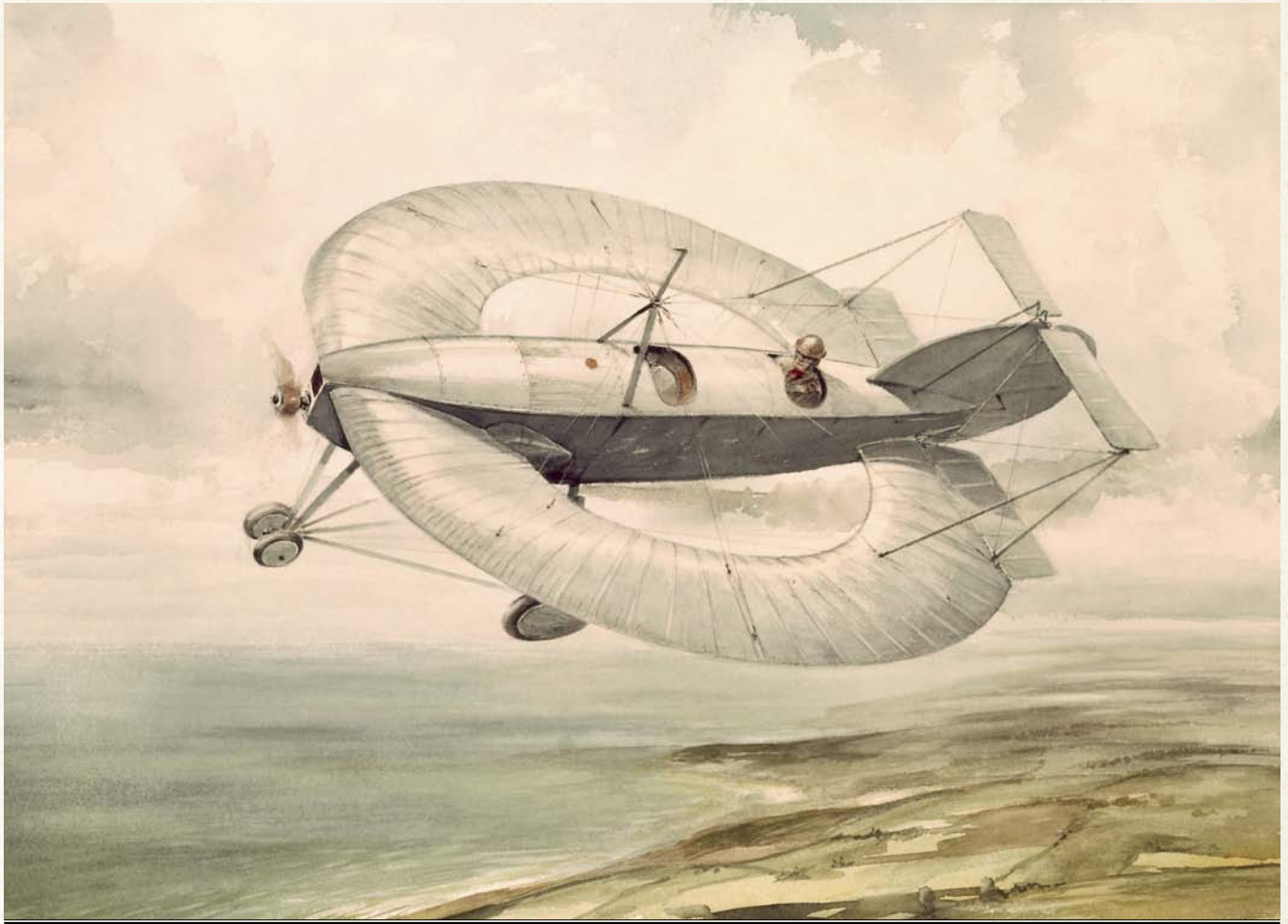
THE PILOT OF THE LEE-RICHARDS ANNULAR MONPLANE SAT IN THE REARMOST OF THE TWO COCKPITS; A PASSENGER SAT IN FRONT
