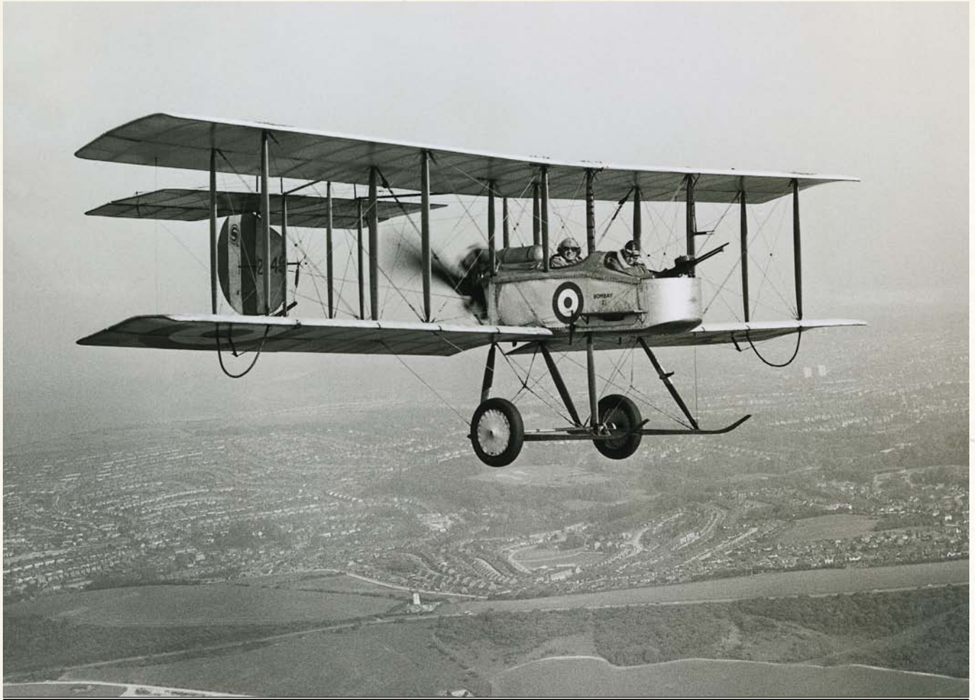
THE PROPELLER OF THE VICKERS F.B.5 WAS SET BEHIND THE WINGS TO ALLOW THE GUNNER, SEATED IN FRONT, A CLEAR FIELD OF FIRE
