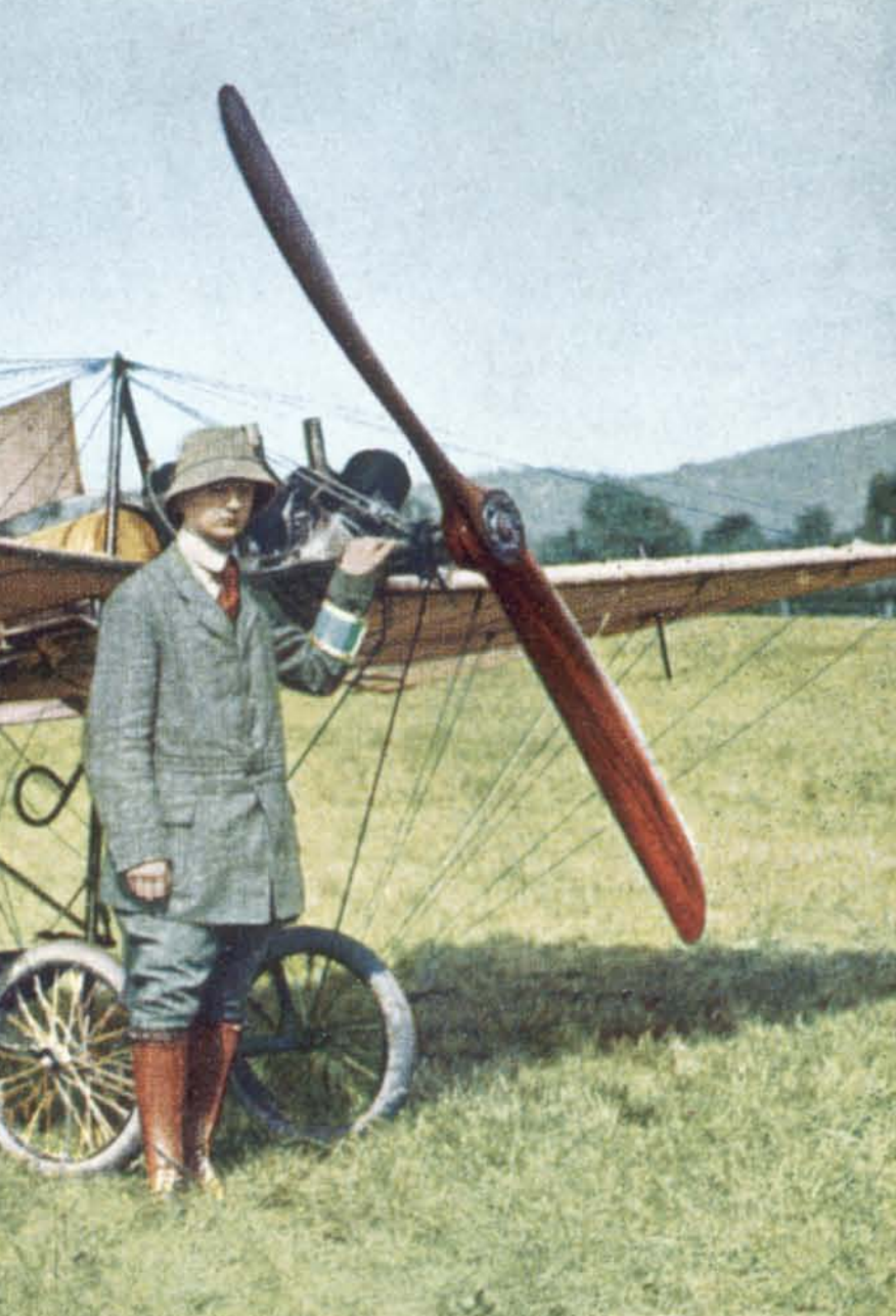
This early colour photograph shows a German Grade monoplane of 1912, with its creator standing alongside. As in the smaller French Demoiselle, the pilot sat beneath the wings, exposed to the blast from the propeller.
