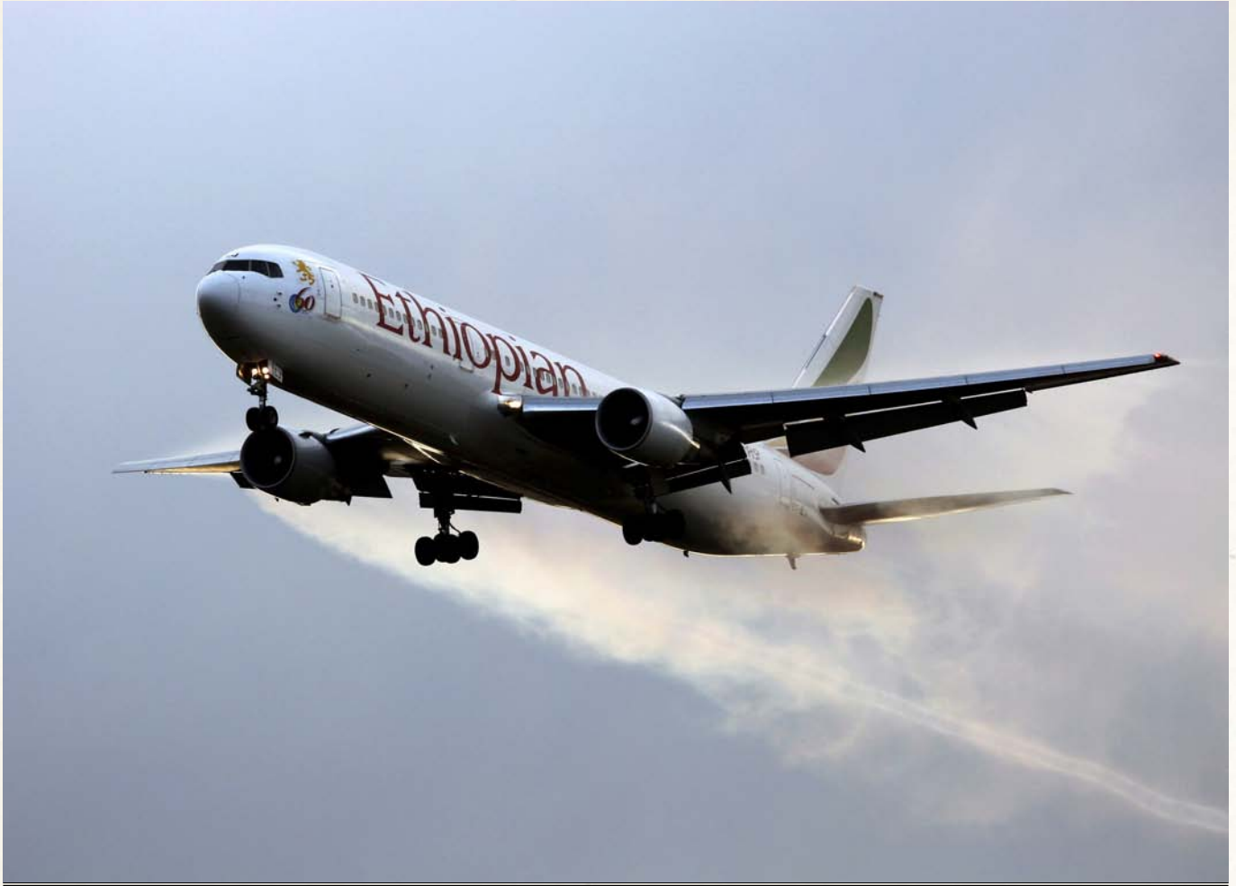
THE BOEING 767 WAS THE FIRST LARGE COMMERCIAL AIRLINER TO FEATURE “RAKED” WINGTIPS, WHICH INCREASE FUEL EFFICIENCY
