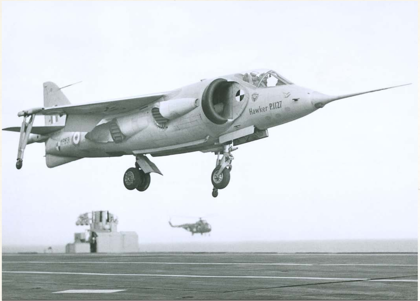
THE P.1127 HAD FOUR ROTATABLE NOZZLES THAT DIRECTED ITS ENGINE EFFLUX VERTICALLY DURING TAKE-OFF AND LANDING
