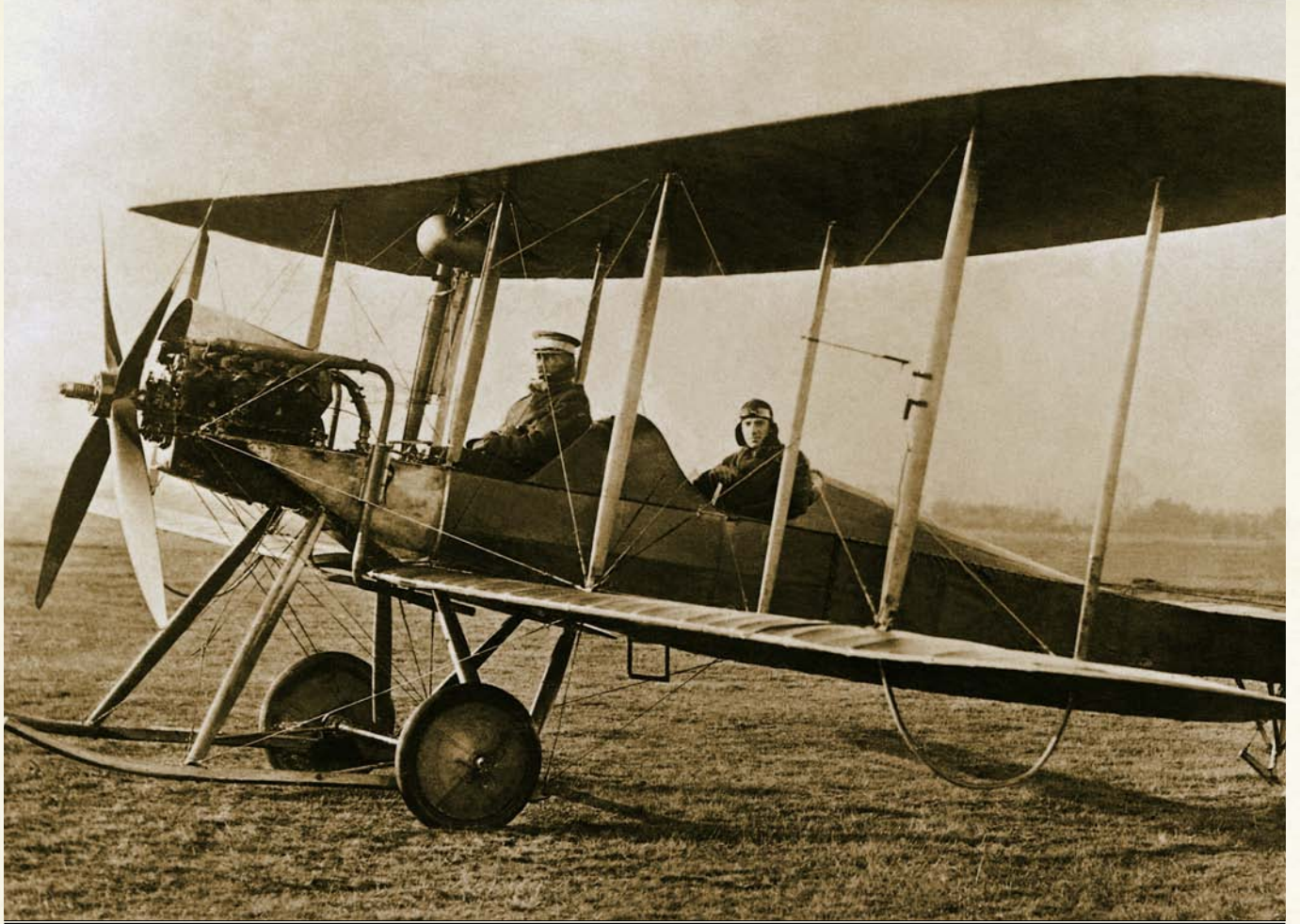
THE B.E.2's MAJOR WEAKNESS WAS ITS STABILITY; MANOEUVRABILITY WAS SACRIFICED, MAKING IT VULNERABLE TO ENEMY ATTACK
