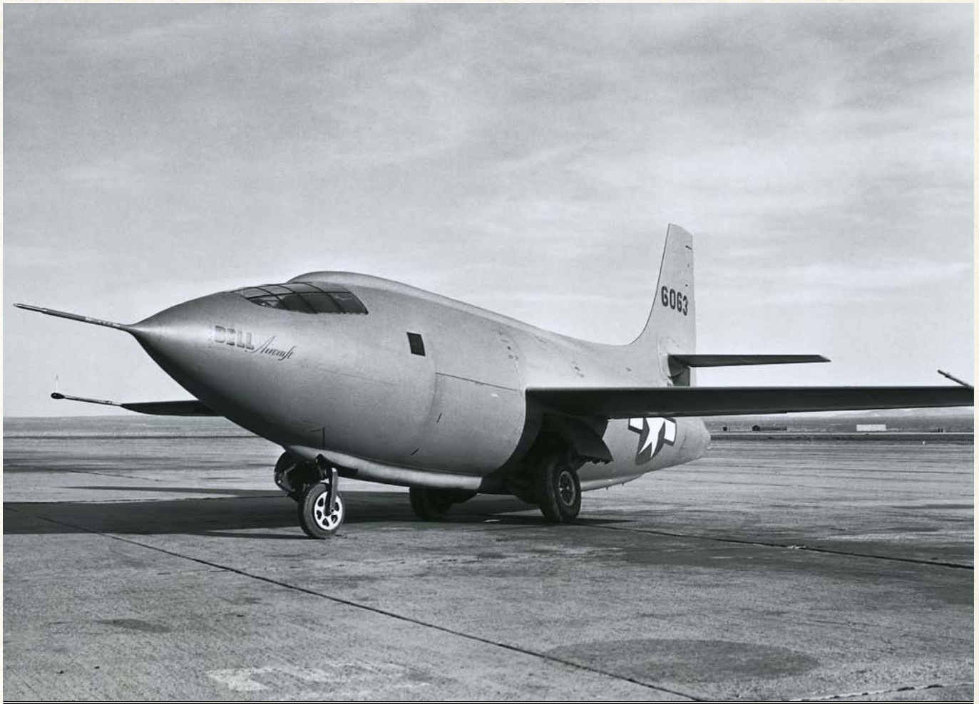
THE SLEEK, AERODYNAMICALLY CLEAN FUSELAGE OF THE SUPERSONIC BELL X-1 RESEMBLED A 0.50-CALIBRE BULLET
