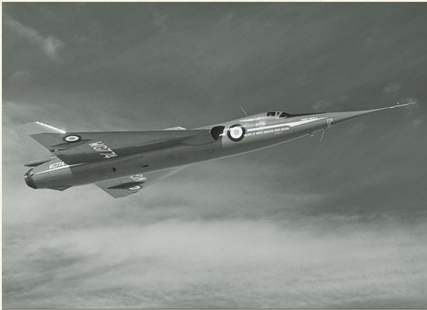
TAILLESS AND WITH A DISTINCTIVE NEEDLE NOSE, THE BRITISH F.D.2 WAS CREATED TO INVESTIGATE TRANSONIC FIGHT
