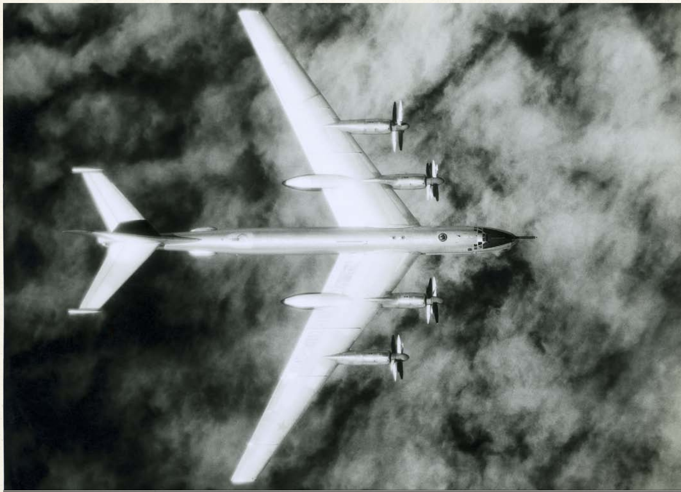
THE WORLD'S ONLY TURBOPROP BOMBER, THE TUPOLEV BEAR COMBINED PROPELLERS WITH THE SWEPT WING OF A JET AIRCRAFT
