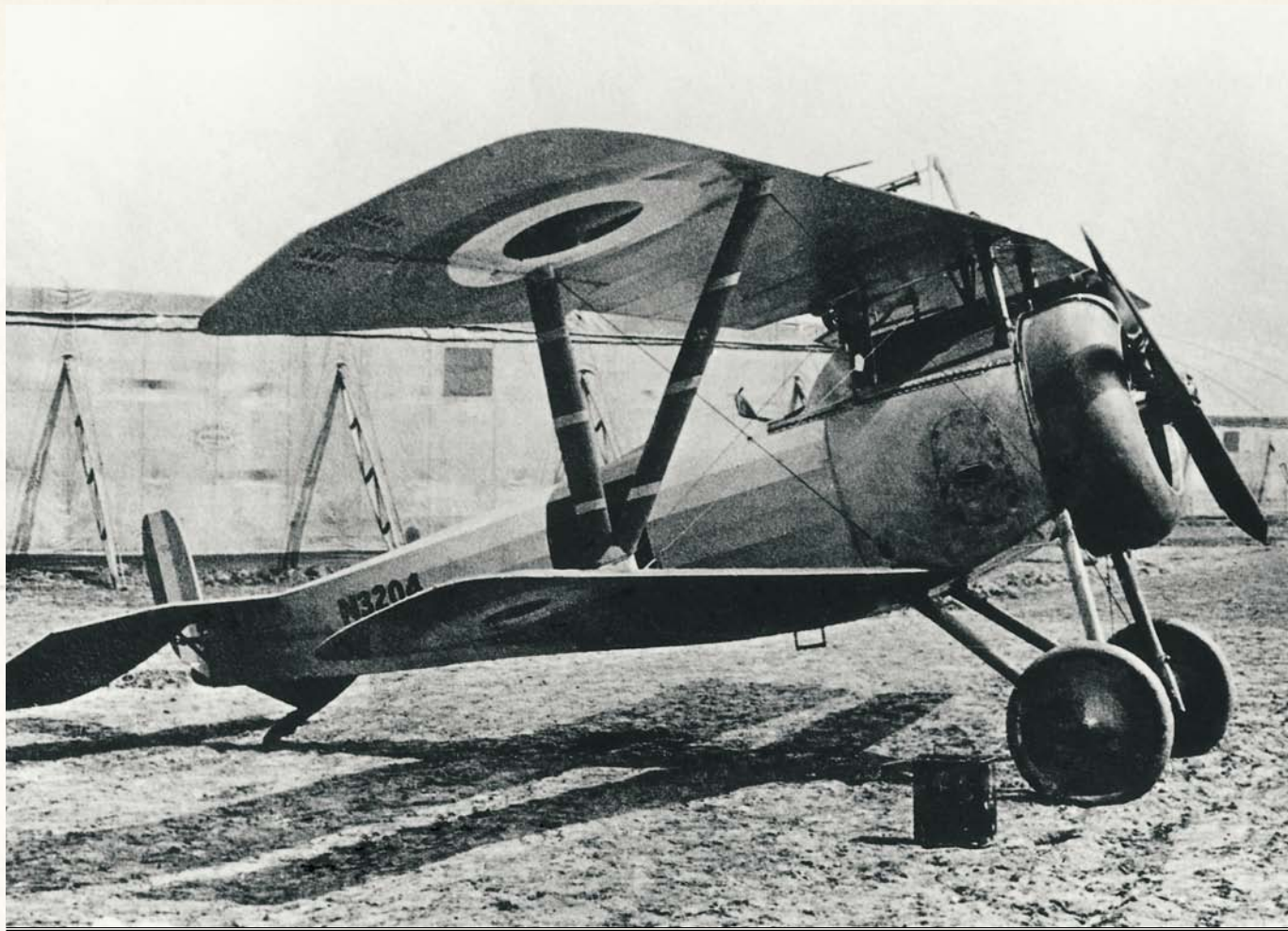
A HIGHLY SUCCESSFUL FRENCH FIGHTER, THE NIEUPORT 17 HAD A DISTINCTIVE LARGE UPPER WING AND A SMALL LOWER WING
