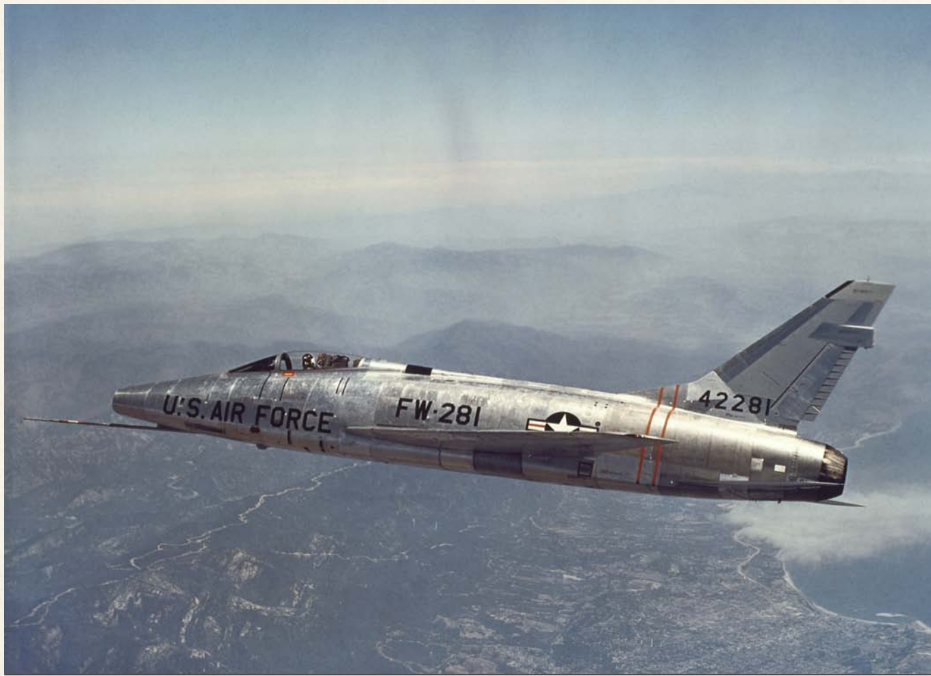
THE SUPERSONIC SUPER SABRE JET FIGHTER HAD A SWEPT WING AND AN UNDERFUSELAGE SPEED BRAKE
