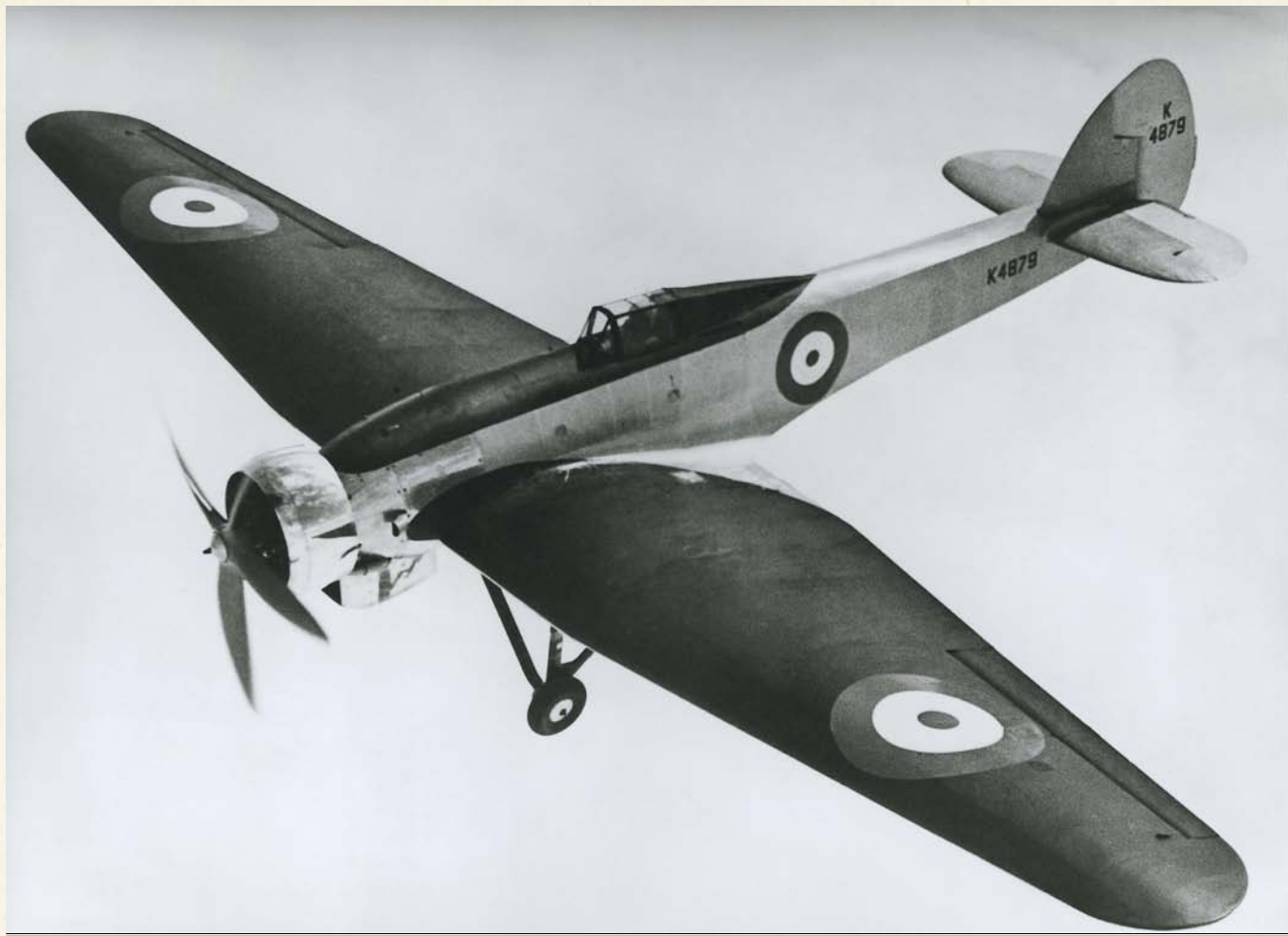
A LIGHTWEIGHT, SLENDER FRAME AND BROAD WINGS EQUIPPED THE TYPE 138A FOR CLIMBING TO PREVIOUSLY UNATTAINED HEIGHTS
