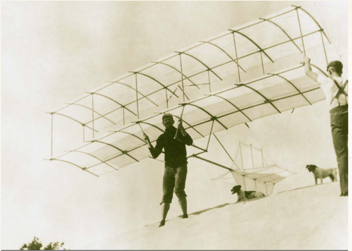
THE OUTSTANDING FEATURE OF CHANUTE'S GLIDER WAS ITS WING STRUCTURE, A RIGID, OPEN "BOX-GIRDER" STILL USED TODAY
