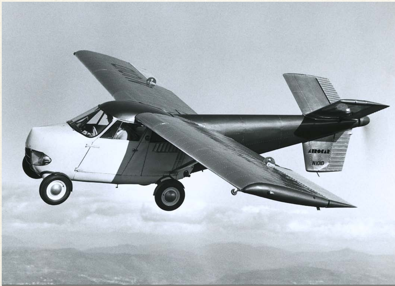
THE AEROCAR COMPRISED A CAR AND A DETACHABLE ONE-PIECE STRUCTURE INCORPORATING WINGS, TAIL, AND PROPELLER
