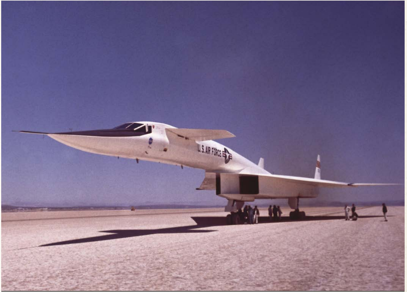
THE XB-70'S SIX POWERFUL ENGINES WERE NEATLY HOUSED IN AN UNDERWING BOX STRUCTURE.
