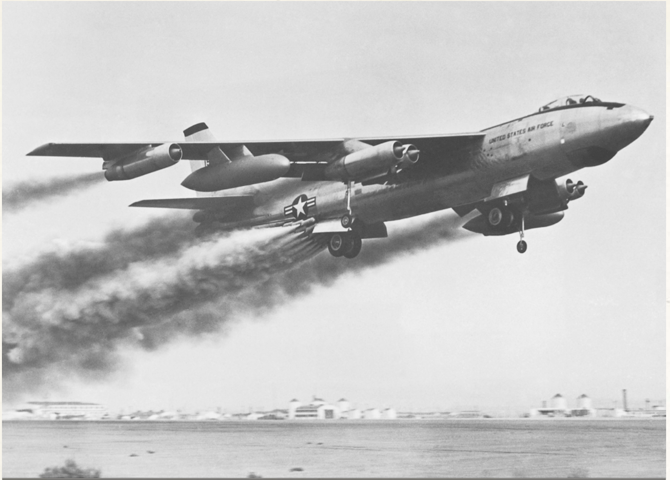
THE EXCEPTIONALLY FAST B-47 BOMBER HAD AN INNOVATIVE SWEEPED WING AND SIX JET ENGINES HOUSED IN UNDERWING PODS
