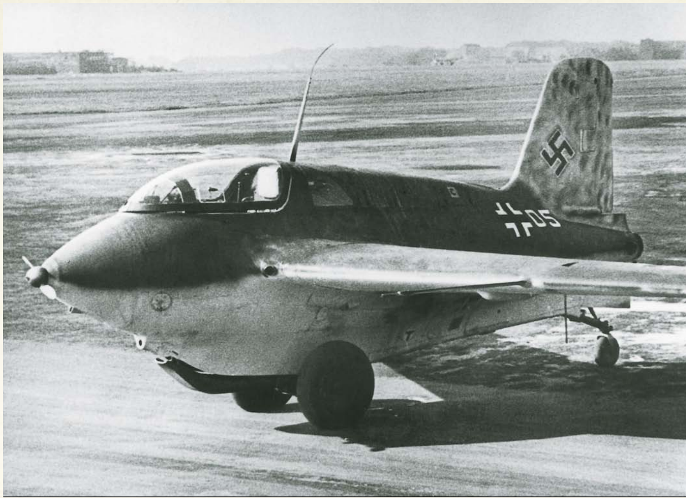
A REVOLUTIONARY ROCKET-POWERED INTERCEPTOR, THE Me 163 KOMET COULD CLIMB WITH PHENOMENAL SPEED
