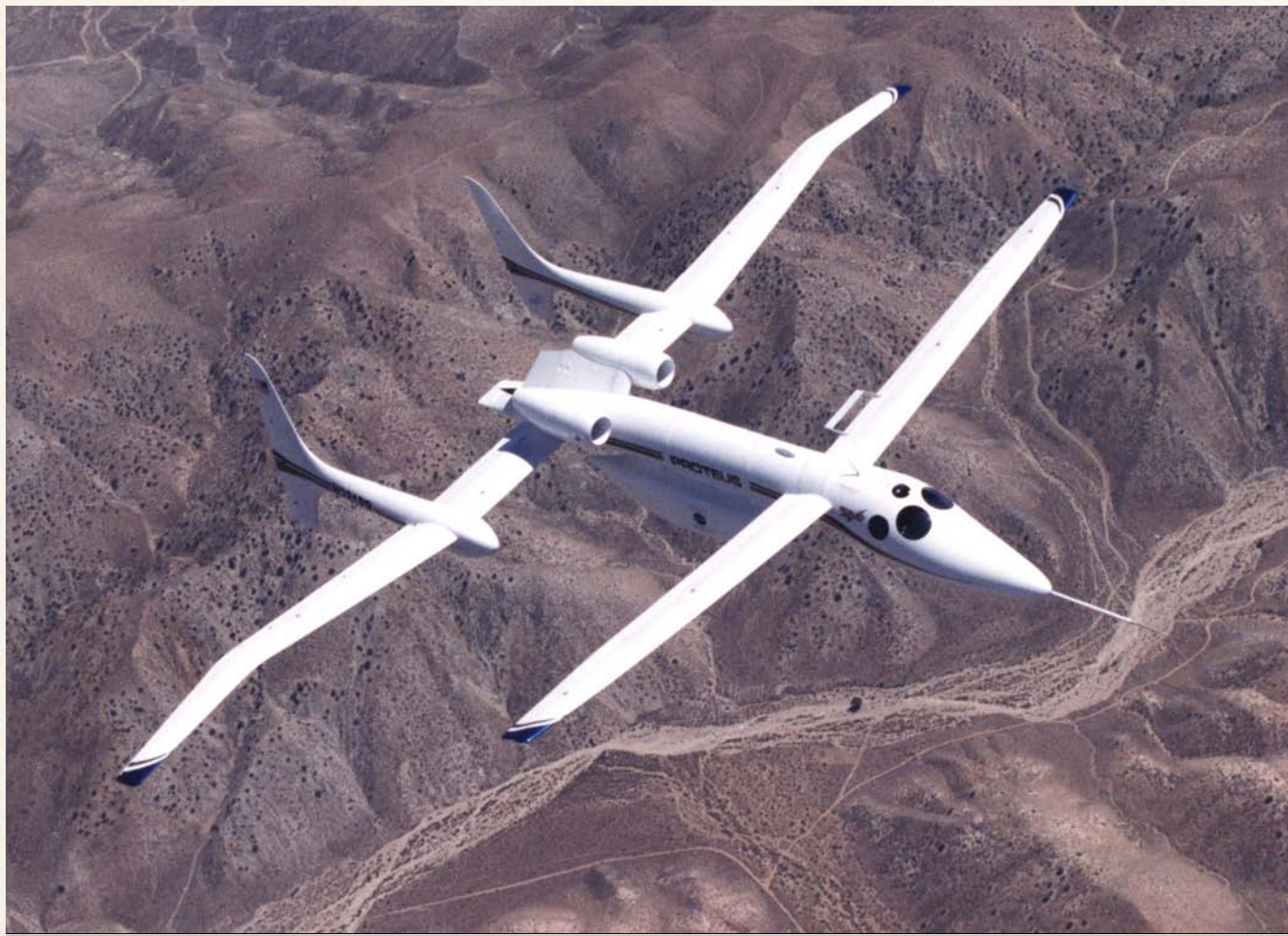
PROTEUS HAS AN UNUSUAL TANDEM-WING AND TWIN-BOOM DESIGN WITH REAR-MOUNTED TURBOFAN ENGINES
