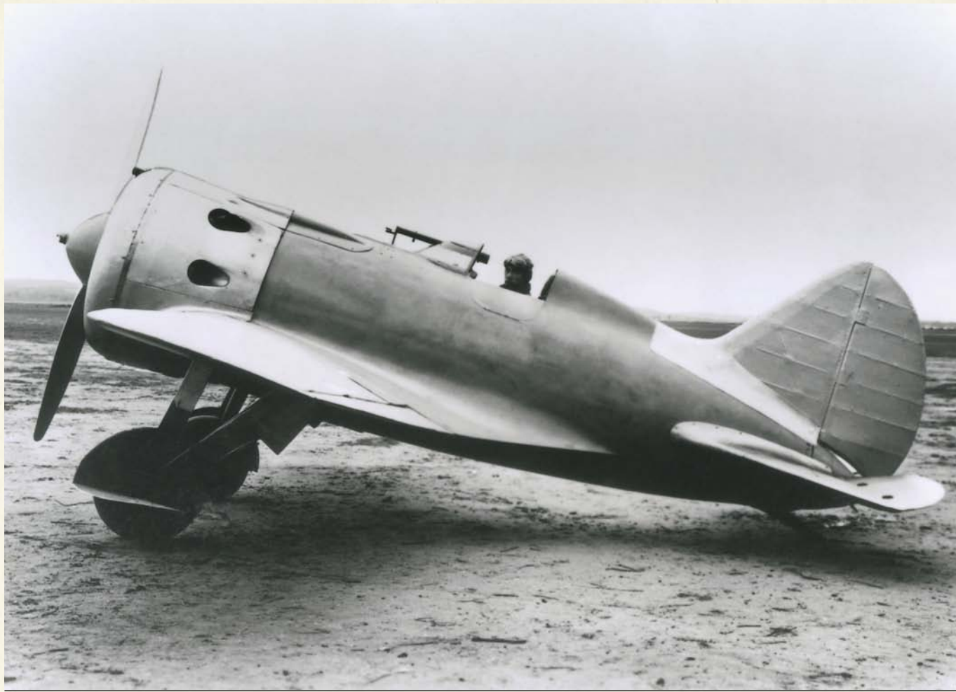
THE "LITTLE DONKEY" WAS A SINGLE-SEAT MONOPLANE FIGHTER WITH A RETRACTABLE UNDERCARRIAGE
