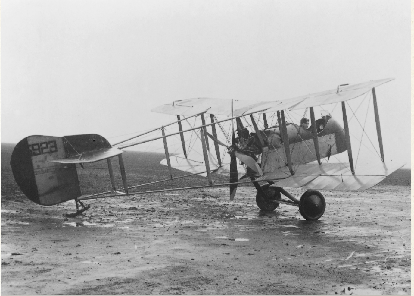
D.H.2 PILOTS FOUND IT DIFFICULT TO CONTROL THE AEROPLANE AND FIRE THE LEWIS GUN AT THE SAME TIME.
