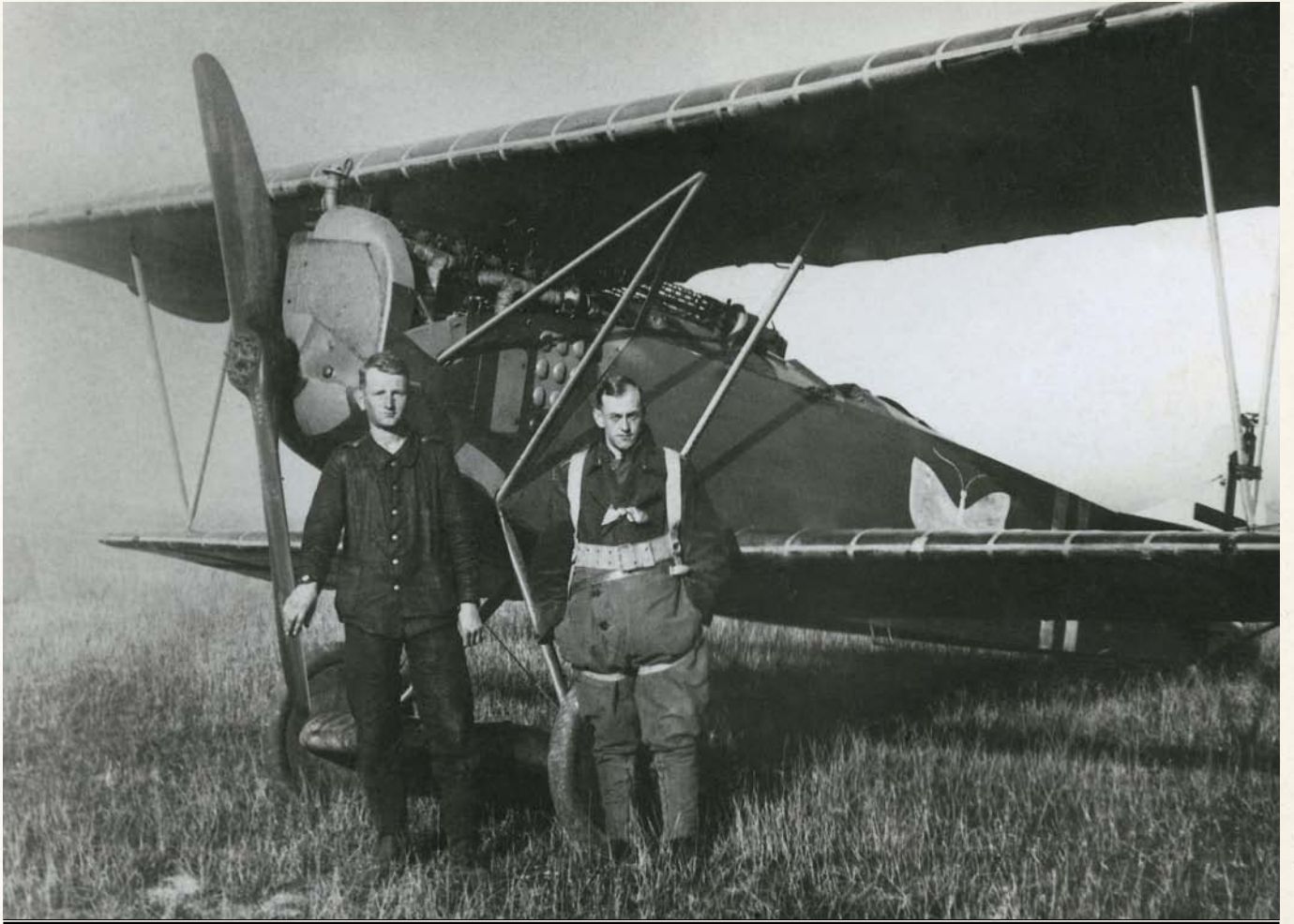
THE D.VII'S INTERPLANE STRUT ARRANGEMENT MEANT THAT BRACING WIRES WERE NO LONGER NECESSARY
