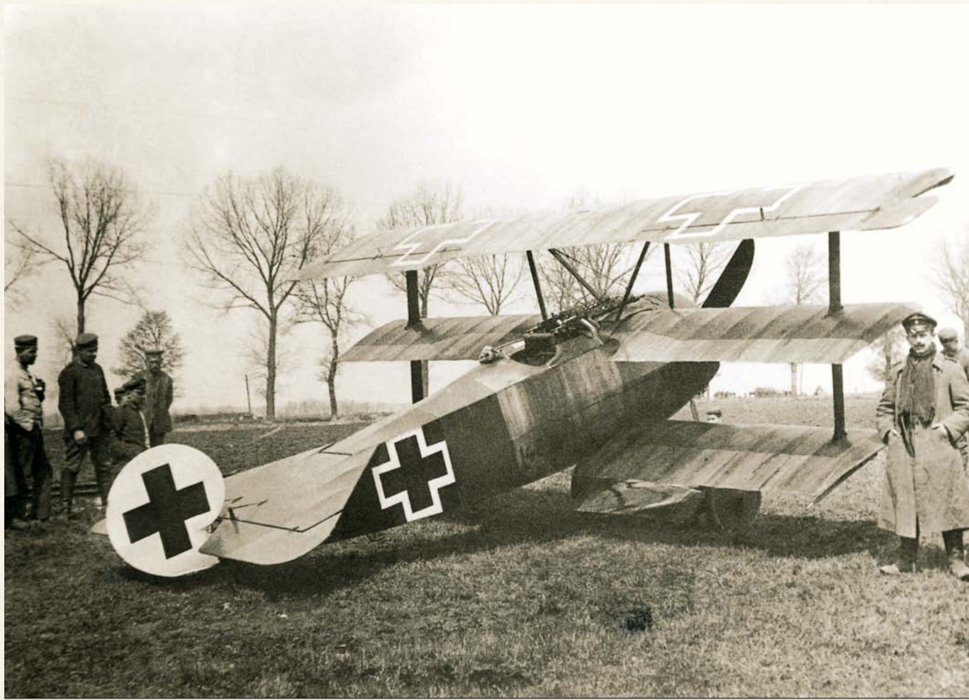
"I" STRUTS WERE ADDED TOWARDS THE Df.1 TRIPLANE'S WINGTIPS TO PREVENT THE WINGS VIBRATING IN FLIGHT
