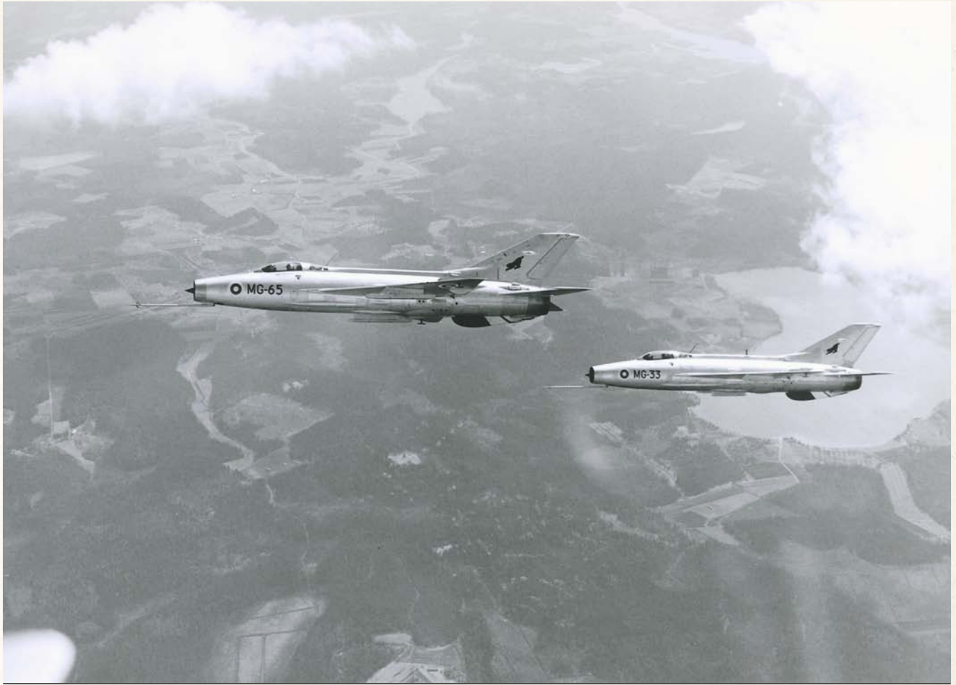
THE AGILE AND SUCCESSFUL MiG-21 WAS A SIMPLE, SINGLE-ENGINE FIGHTER ARMED WITH JUST TWO MISSILES AND A CANNON
