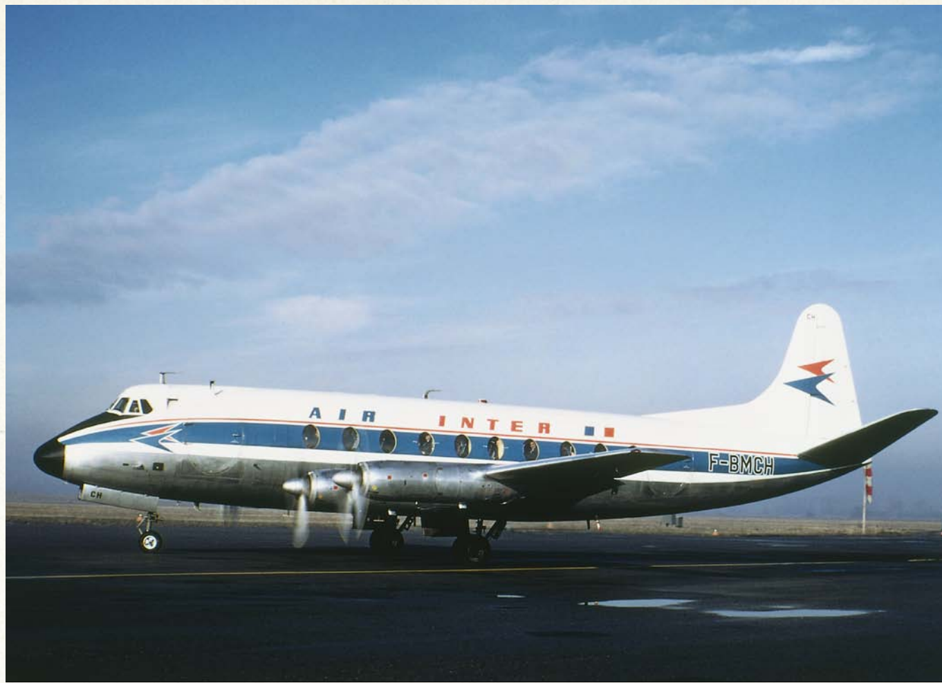
THE HUGELY POPULAR VISCOUNT WAS THE FIRST TURBOPROP AIRLINER; IT WAS QUIETER AND FASTER THAN PISTON-ENGINE PLANES
