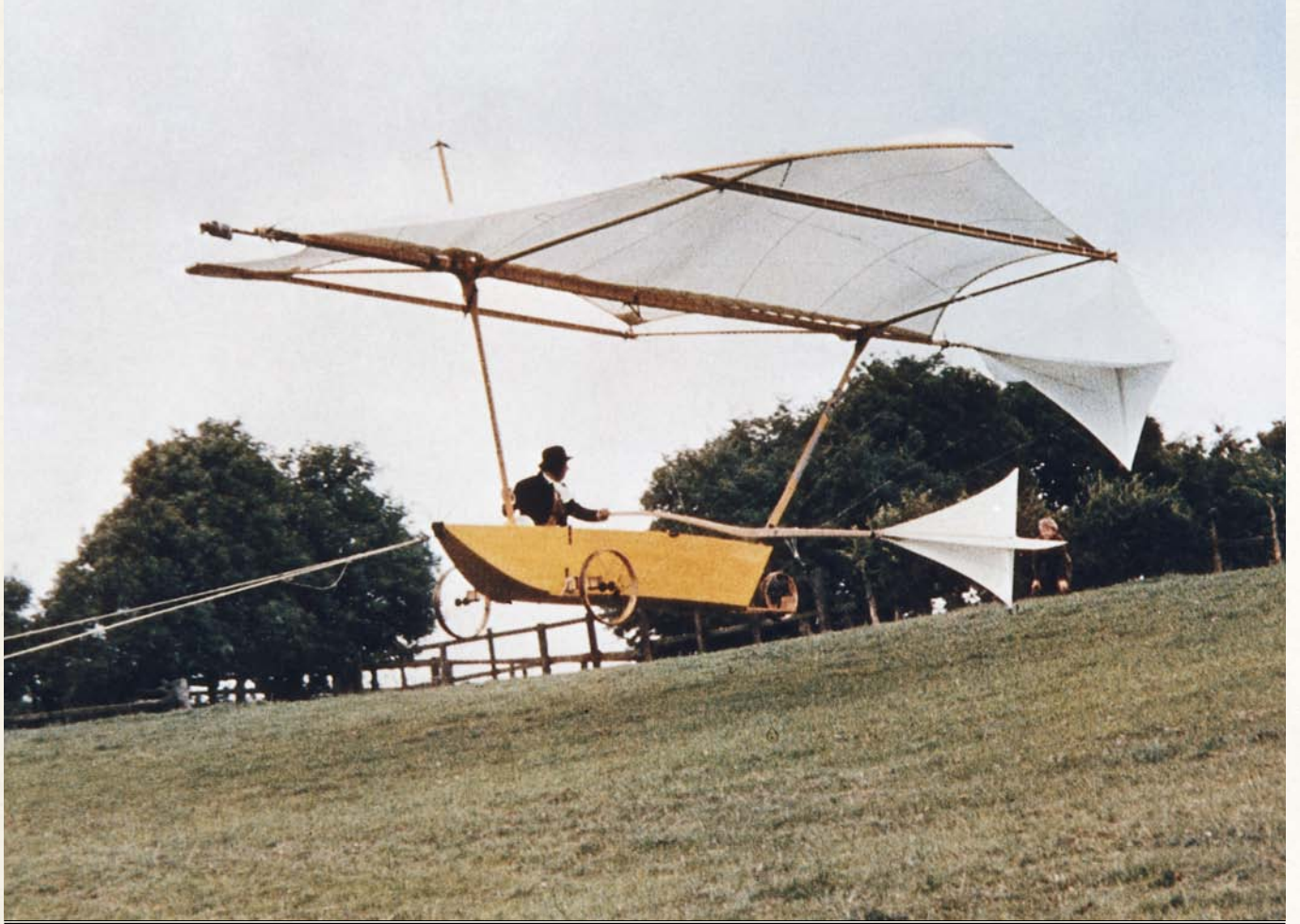
CAYLEY'S GLIDER HAD A BOAT-LIKE FUSELAGE AND AN UNDERCARRIAGE SPORTING INGENUOUS, TENSION-SPOKED WHEELS
