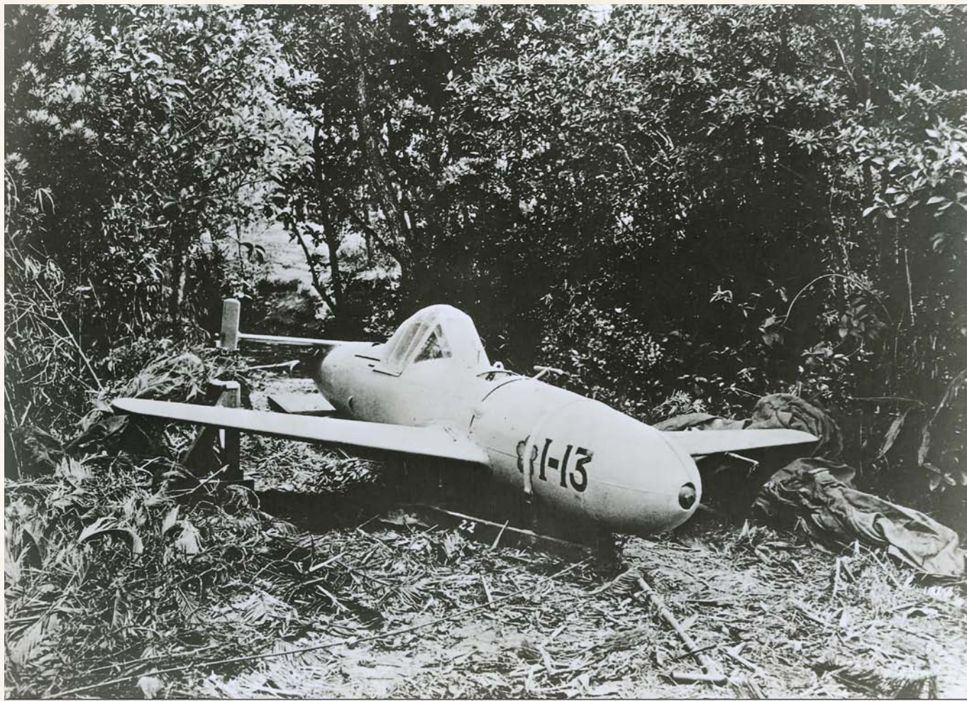
CHEAPLY PRODUCED, THE OHKA WAS A SINGLE-SEAT, ROCKET-PROPELLED FLYING BOMB PILOTED BY JAPANESE KAMIKAZE PILOTS
