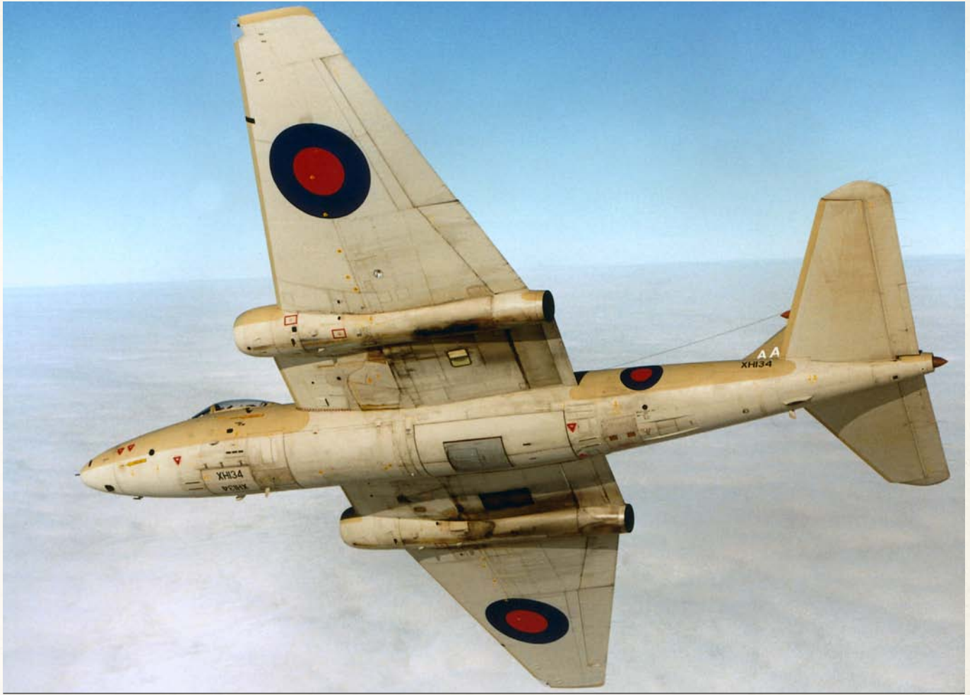
THE CANBERRA WAS SO FAST THAT IT WAS NOT EQUIPPED WITH DEFENSIVE WEAPONS; THIS IS A PHOTO-RECONNAISSANCE VARIANT
