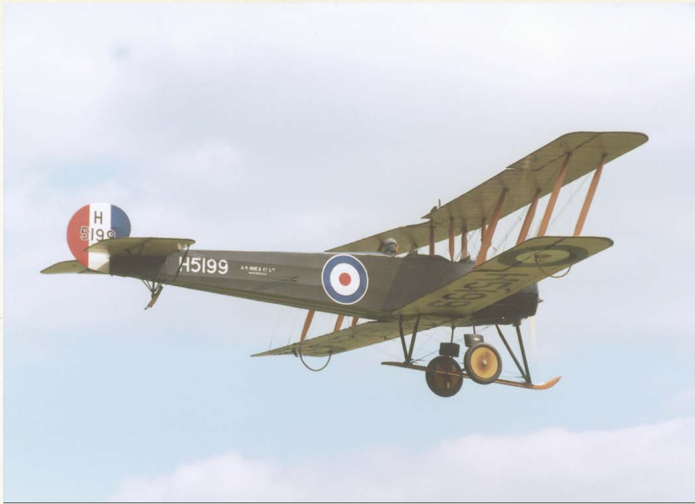
WITH ITS DISTINCTIVE, COMMA-SHAPED RUDDER, THE AVRO 504 WAS THE AEROPLANE IN WHICH MANY EARLY PILOTS LEARNED TO FLY
