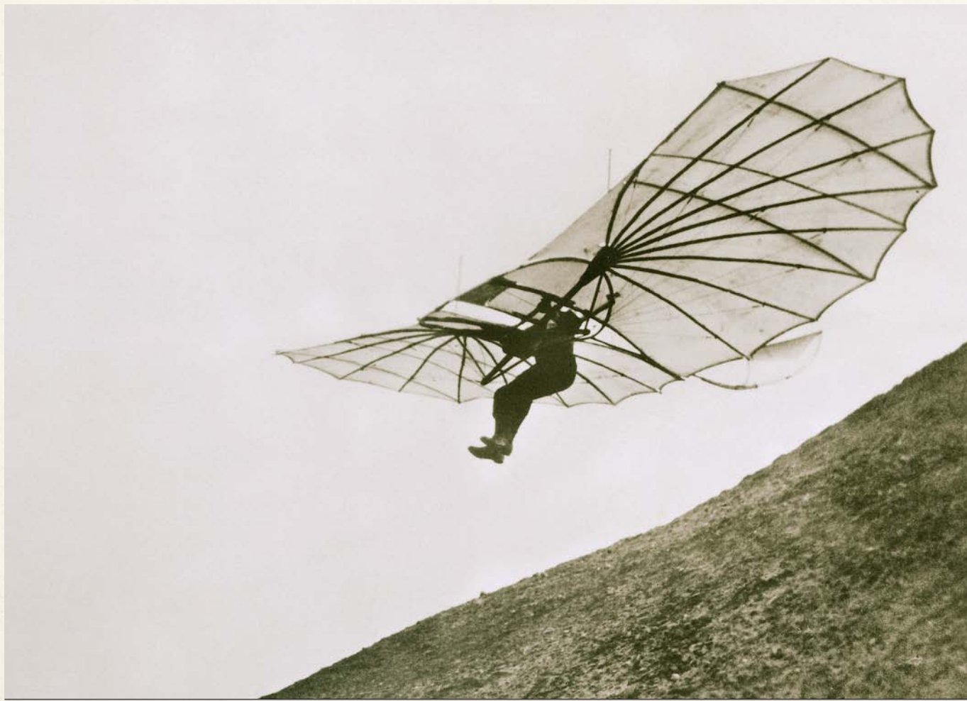
LILIENTHAL'S NO.11 HANG-GLIDER WAS CONTROLLED BY SIMPLY SWINGING THE BODY BACK AND FORTH
