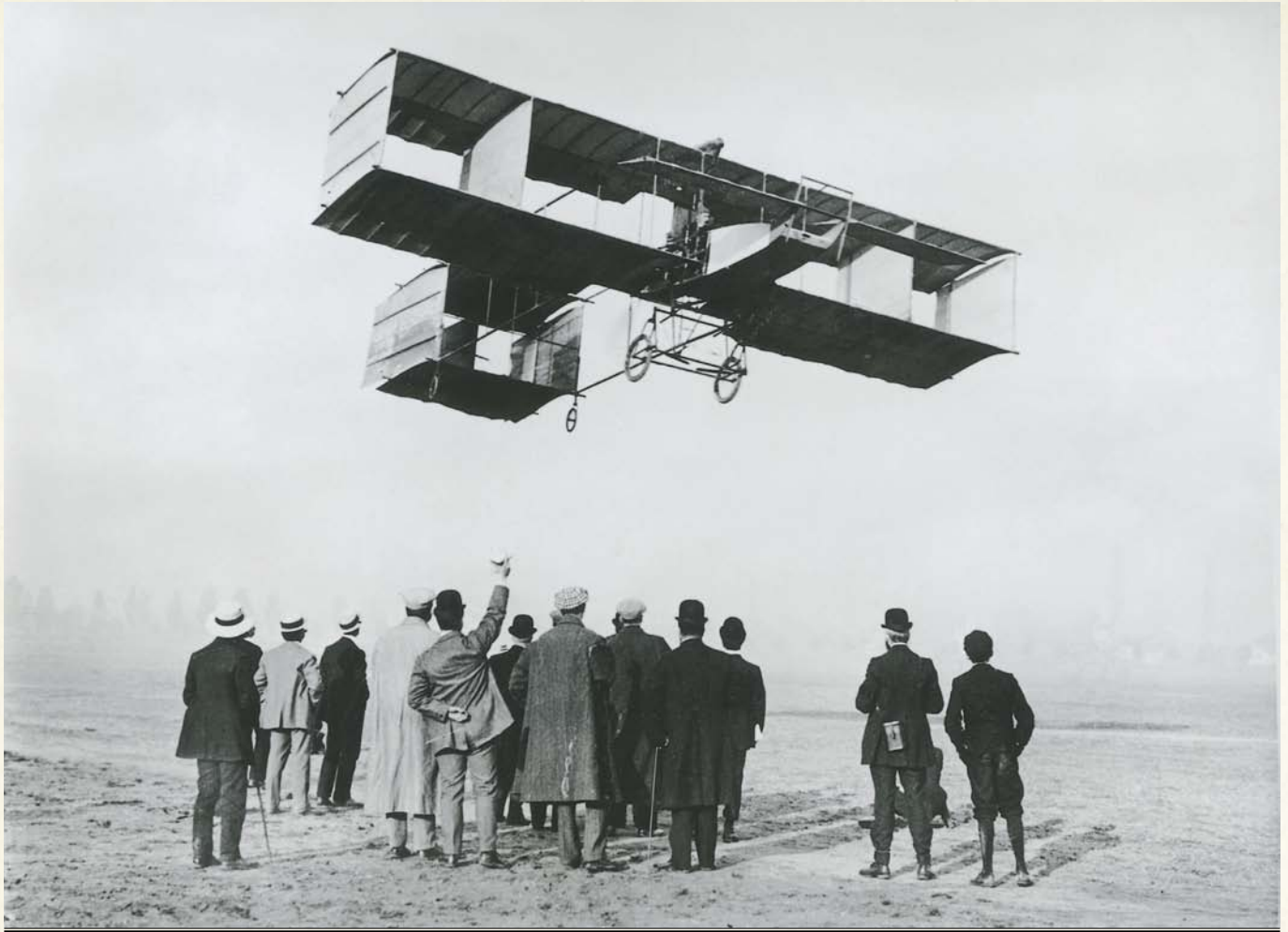
THE VOISIN BIPLANE RELIED ON RUDDER CONTROL, SO TURNS HAD TO BE FLAT AND WIDE TO AVOID SIDESLIPPING INTO THE GROUND
