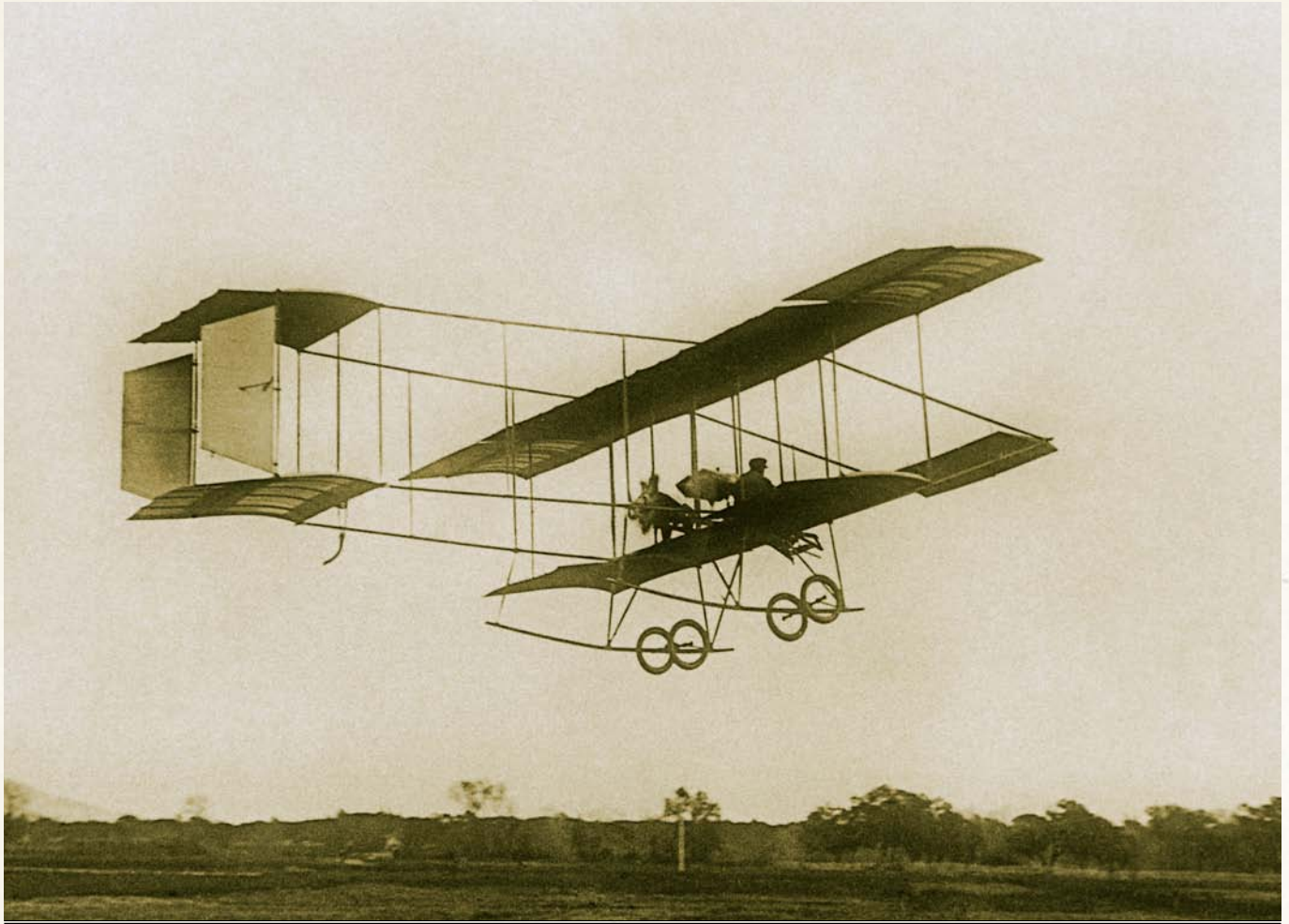
EASY TO FLY AND WITH A GOOD REPUTATION FOR SAFETY, THE FARMAN III WAS THE CLASSIC PRE-WORLD WAR I BIPLANE
