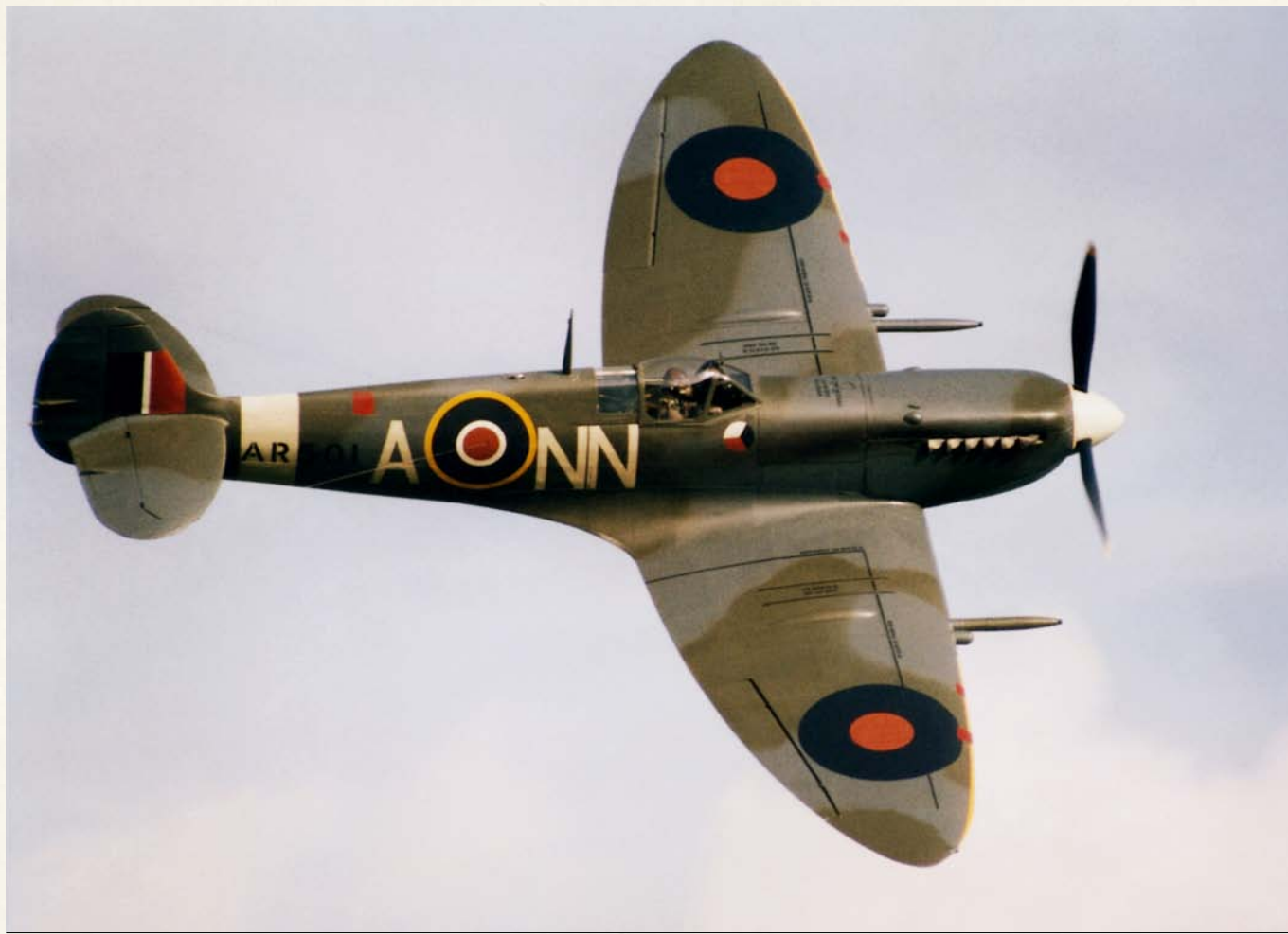
THIN WINGS, A SMALL FUSELAGE SECTION, AND REFINED STREAMLINING MADE THE SPITFIRE BOTH ELEGANT AND FAST
