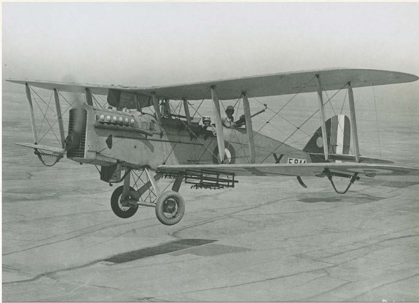
THE D.H.9A'S PILOT'S AND OBSERVER'S COCKPITS WERE CLOSER TOGETHER THAN IN THE D.H.4, MAKING COMMUNICATION MUCH EASIER
