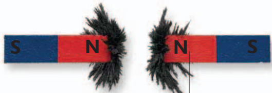
Similar poles of a magnet repel each other.
