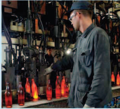
Glass bottles are shaped from molten glass.
