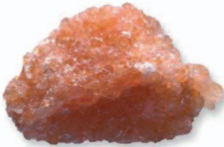
Rock salt is a mineral that is spread on roads in icy weather. It makes the ice melt.
