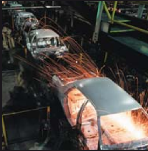
Robots join the car parts together with welding torches.
