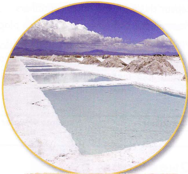
Salt works are used to extract salts from seawater using evaporation.
