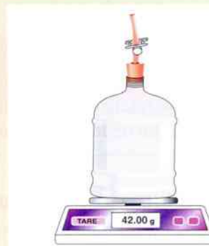
The plastic container is weighed when it is full of air, and when the air has been pumped out.
