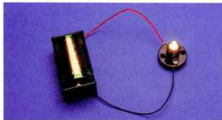
An electric current makes the lamp light up.
