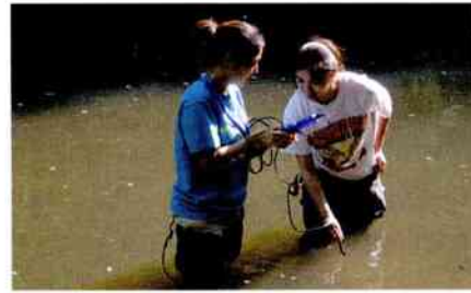
The students use an oxygen meter to measure the concentration of dissolved oxygen in the water.
