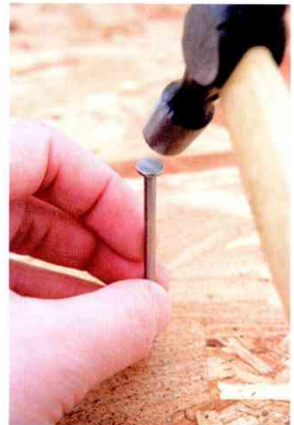
Hammering a nail.
