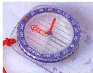
The red end of the compass needle points towards the north.
