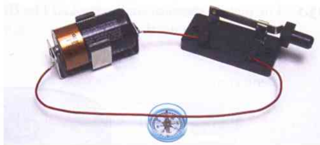
A current in the wire makes a magnetic field.
