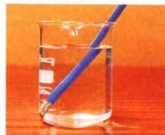
The pencil looks broken – we see the lower half of it through water.
