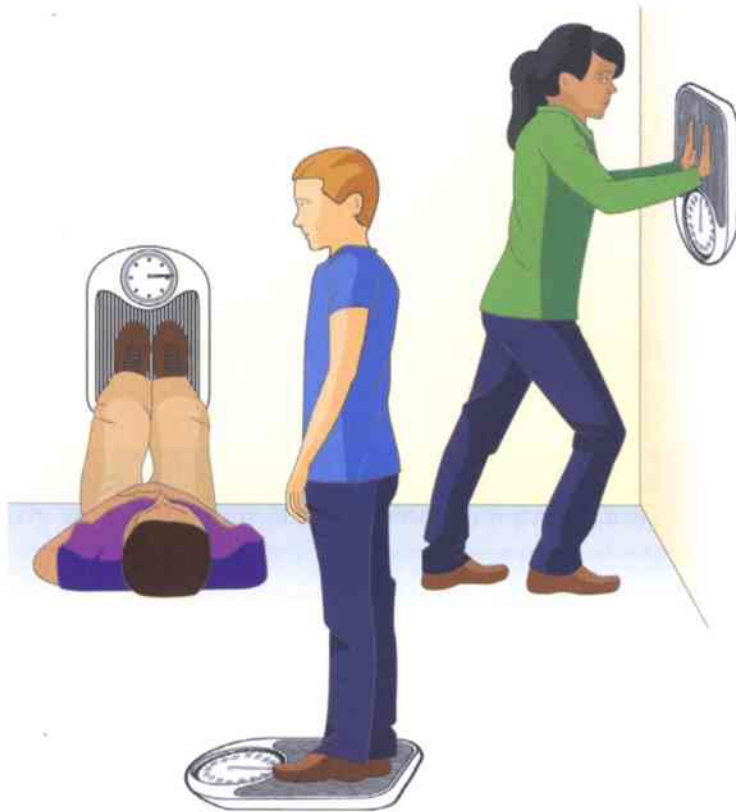
Weighing scales can be used to measure a pushing force.
